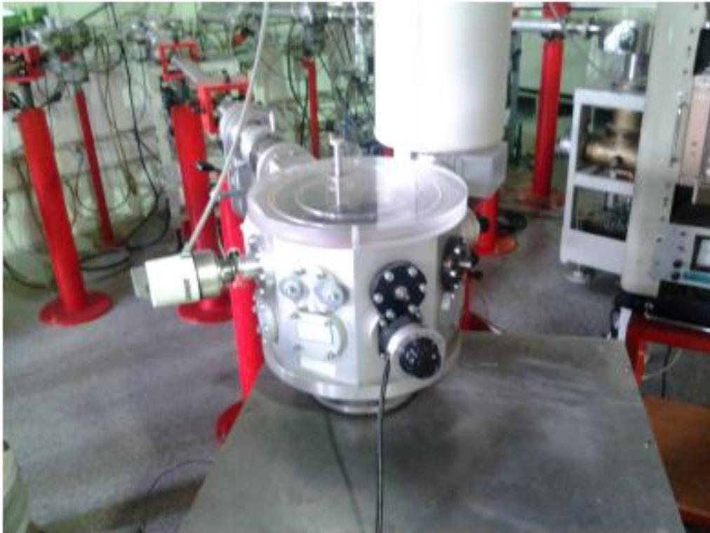
**Fig 1: Schematic of the ion beam, target, and detector arrangement in the PIXE chamber used for measurements**
