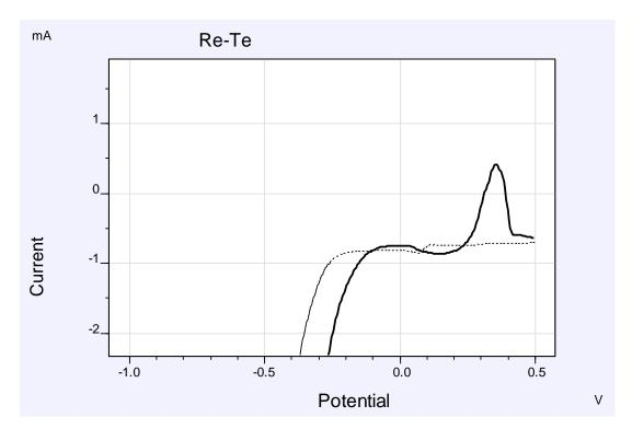
Fig.3. Volt-ampere cyclic polarizing curves of Re-Te alloy from chlorid solutions on the platinum electrode in the electrolyte contest, mol/l: 7·10<sup>-</sup>3KReO<sub>4</sub>+1,25·10<sup>-2</sup>TeO<sub>2</sub>+2HCl <sub>at</sub> t=75°; V=0,005V/S; pH=0,4
