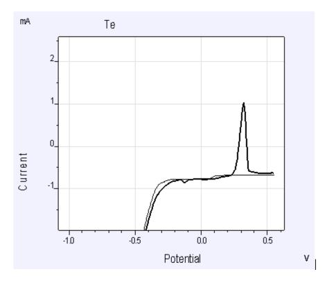
Fig.2. Volt-ampere cyclic polarizing curves of tellurium from chlorid solutions on the platinum electrode in the electrolyte contest, mol/l:  $0.6 \cdot 10^{-2}$ TeO<sub>2</sub>+2HCl at t=75°; V=0.005V/S; pH=0.4
