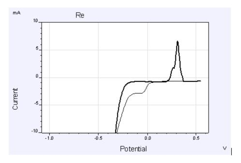
Fig.1. Volt-ampere cyclic polarizing curves of rhenium from chlorid solutions on the platinum electrode in the electrolyte contest, mol/l: 3,5·10<sup>-3</sup>KReO<sub>4</sub>·2HCl at t=75°; V=0,005V/S; pH=0,4
