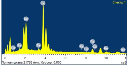
Fig 4. Analysis SEM for obtained thin films in the system Re-Te during 1800 seconds on the platinum
