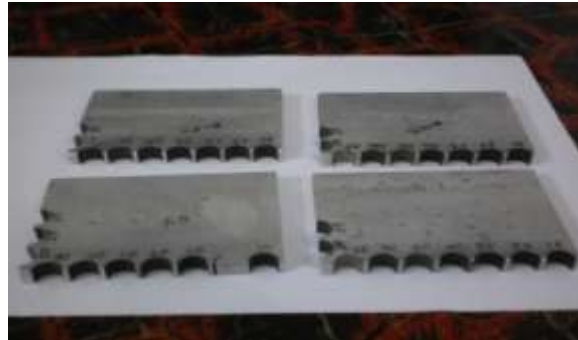
Fig.5b. AA6063/SiC Plate after machining
