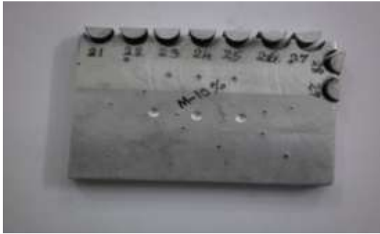
Fig.5a. AA6063/SiC Plate shows circular contour
