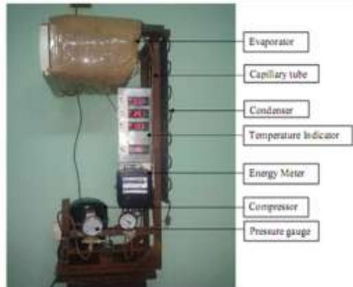
Fig. 1 Schematic of the investigation unit and Apparatus
