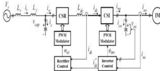
Fig.1 Field oriented control Current source inverter drive system
