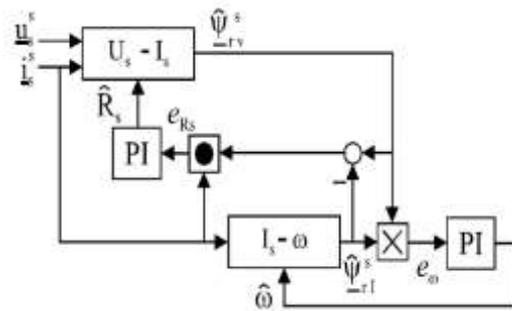
Fig. 4. Proposed MRAS based parallel estimation of rotor speed and stator resistance.
