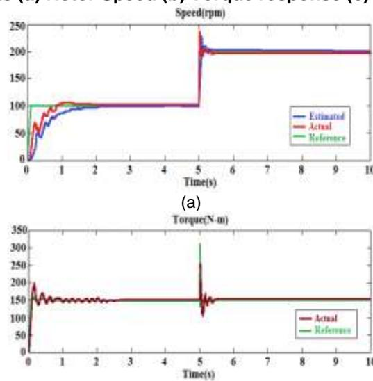
Fig.7 Simulation results (a) Step Speed response (100 to 200rpm) (b) Torque response with Rs compensation
