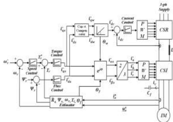
Fig. 3. Structure of the speed sensor less current-fed rotor flux oriented induction motor drive
