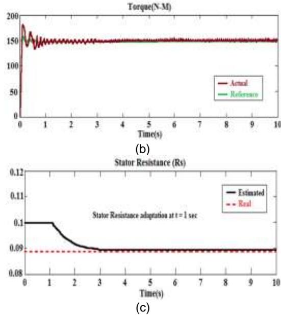
Fig.6 Simulation results (a) Rotor Speed (b) Torque response (c) Rs Estimation(=1.2\*Rs)
