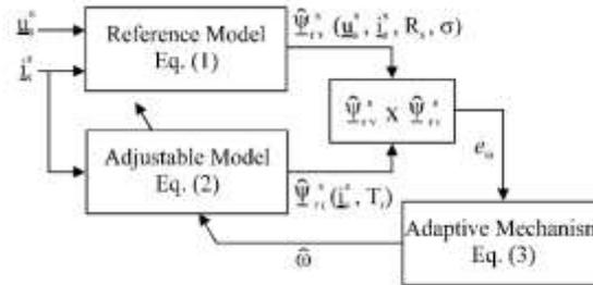
Fig. 2. Basic configuration of the rotor flux based MRAS speed estimator
