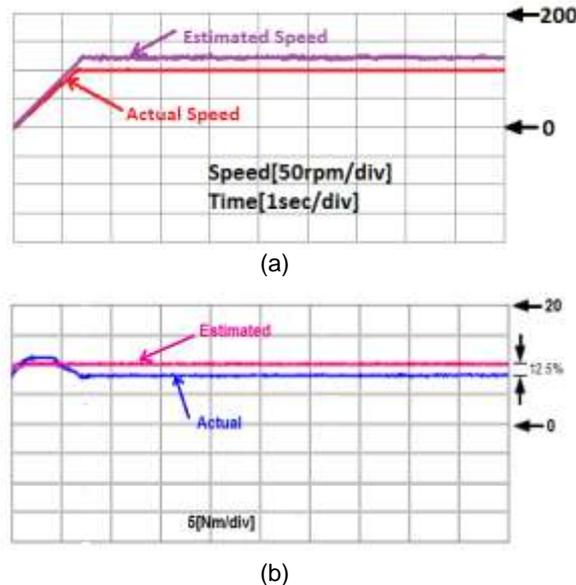
Fig 9 Experimental results without  $R_s$  compensation (a) Rotor Speed (ramp input) with 100rpm
