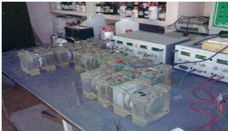
Fig1: RCPT test set –up and apparatus used in this study
