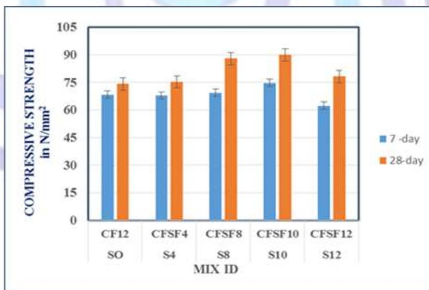
Fig 2: Effect of variation of silicafume on compressive strength of ternary mixes
