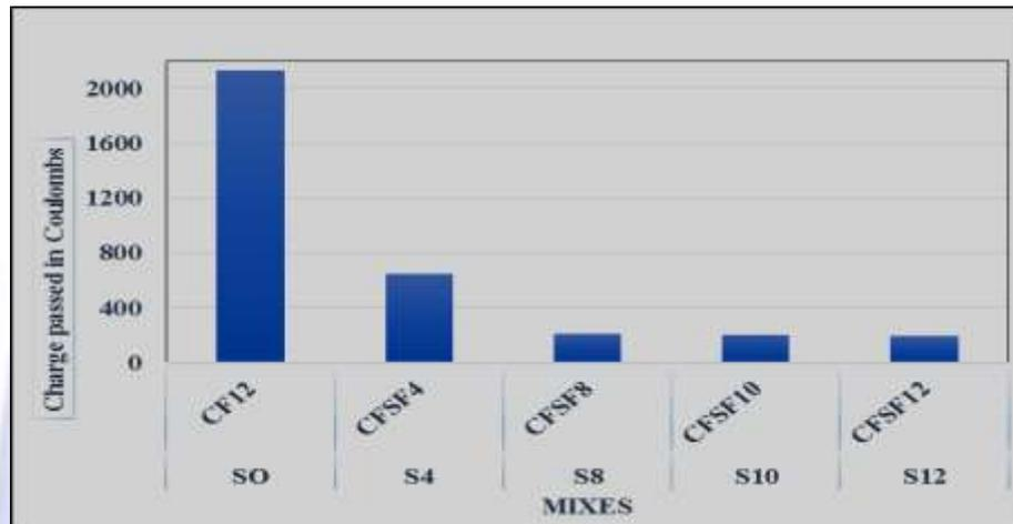
Fig 3: Chloride penetrating rate of ternary mixes having various percentage of silicafume
