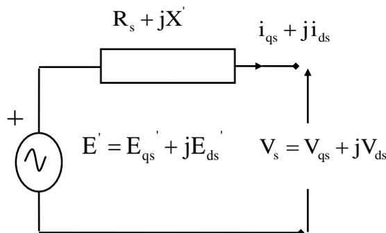
**Fig.2. Thevenin's equivalent circuit of SCIG**
