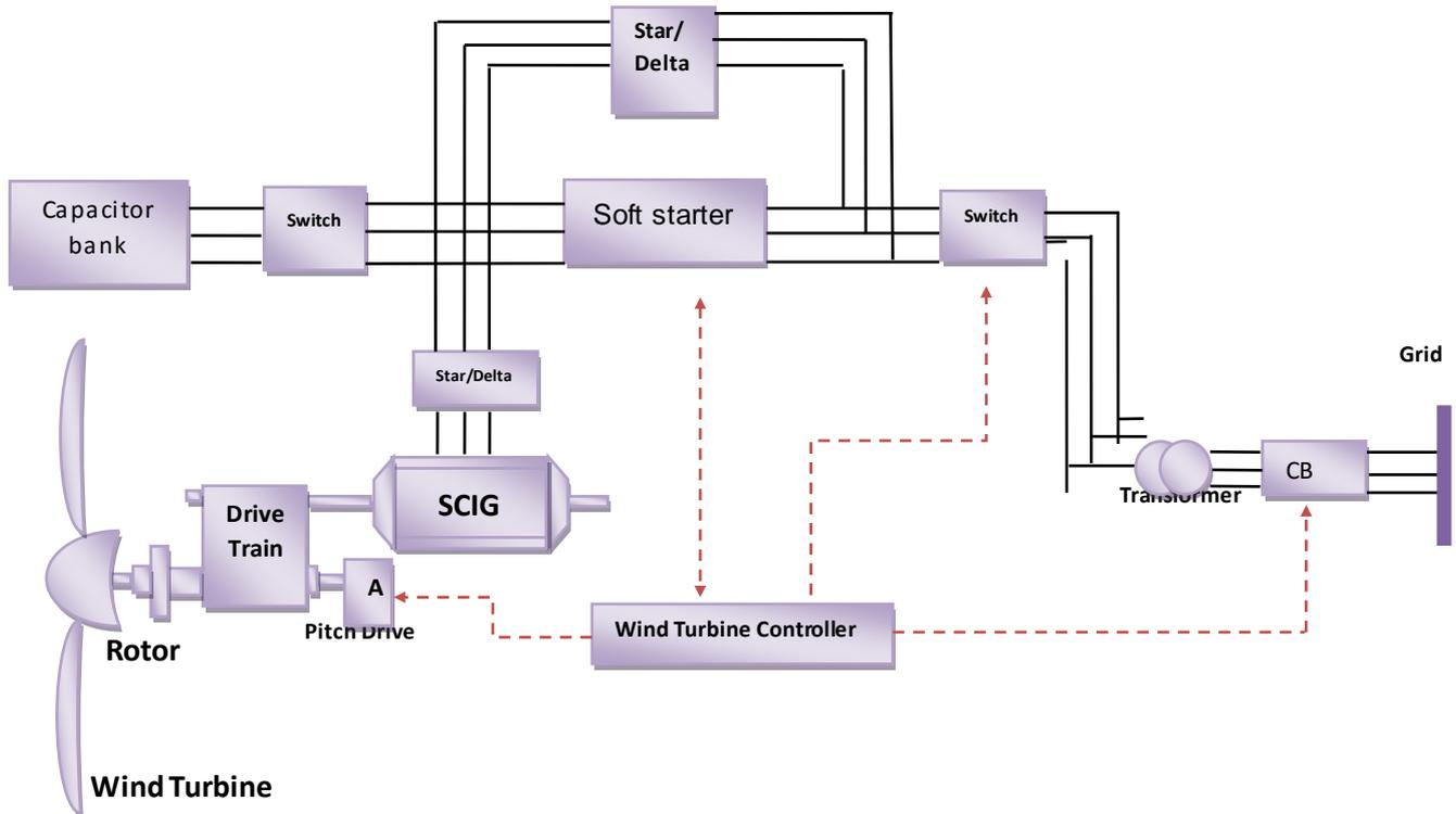
**Fig.1 General structure of fixed speed wind turbine generator**
