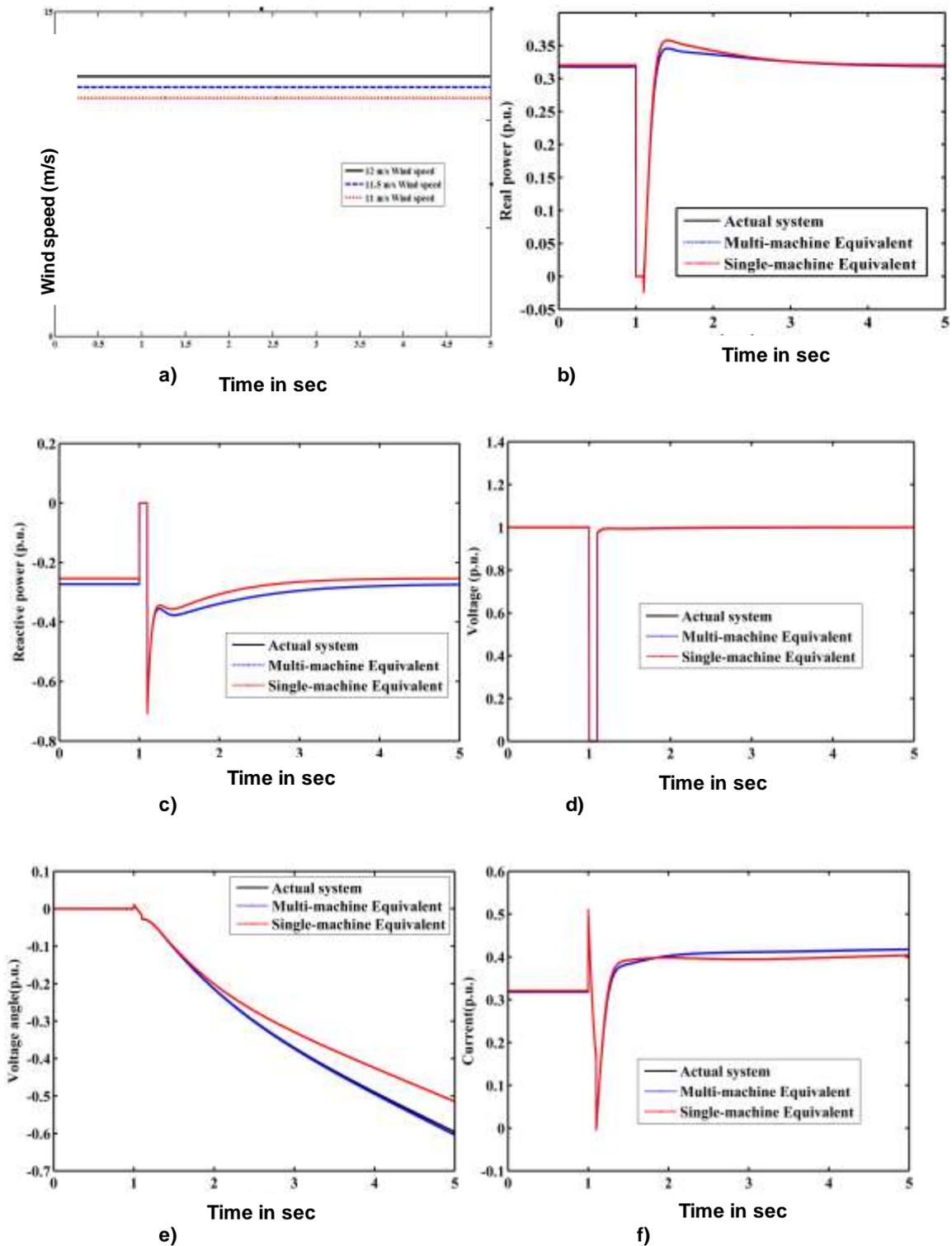
**Fig.6. Actual, multi-machine and single-machine equivalent system responses at the BUS 1 (PCC) during three phase to ground fault a) wind speed curve b) Response of real power c) Response of reactive power responses d) Voltage response e) voltage angle response f) Response of current**
