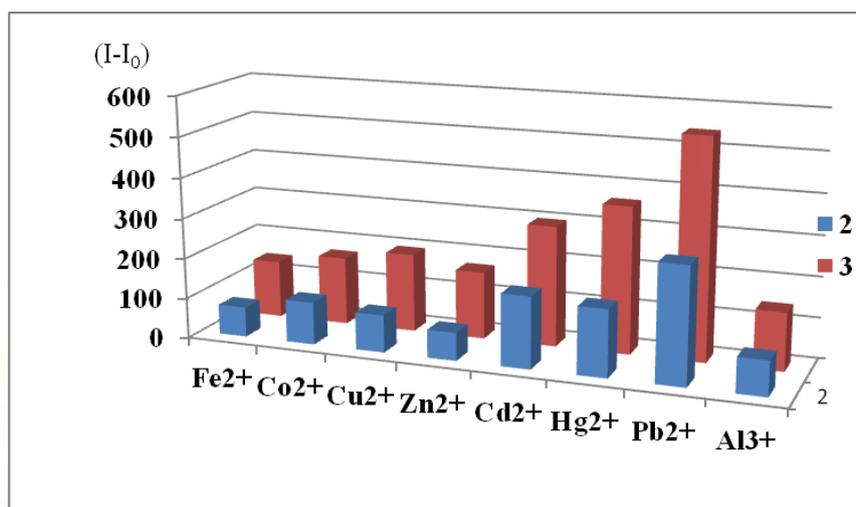
FIGURE 1. Fluorescence changes ( $I - I_0$ ) of **2** and **3** upon the addition of various metal cations<sup>a</sup>
