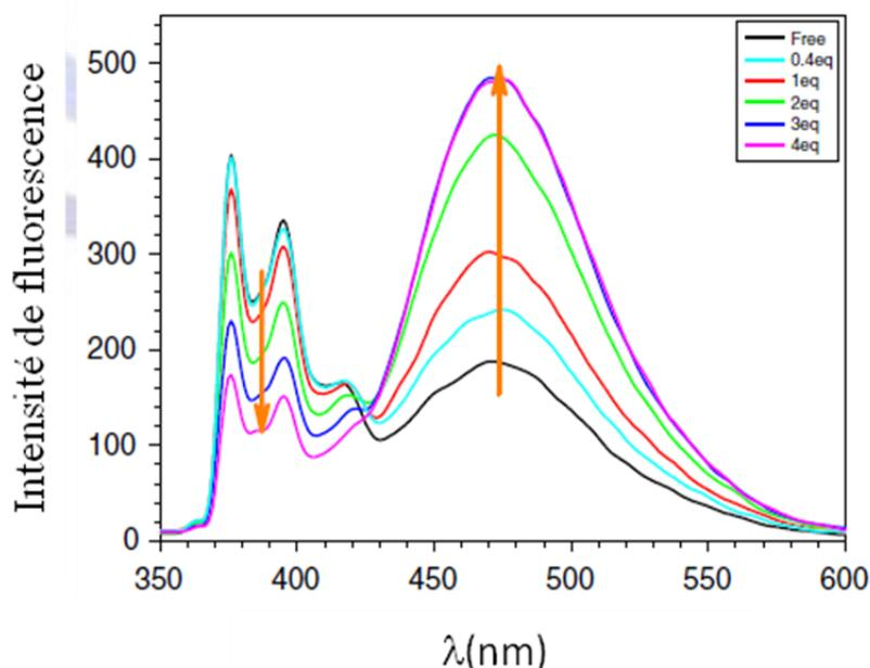
Figure 2. Fluorescence spectra of **3** ( $5.0 \mu\text{M}$ ) in  $\text{CH}_3\text{CN}$  upon addition of increasing concentrations of  $\text{Pb}(\text{ClO}_4)_2$  ( $0 \leq R_{\text{M/L}} \leq 3$ ) with an excitation at  $340 \text{ nm}$
