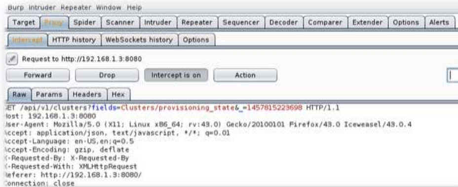
Figure4: HTTP GET request viewed through Burp Suite proxy returned to Machine A from Ambari web portal on Machine B.
